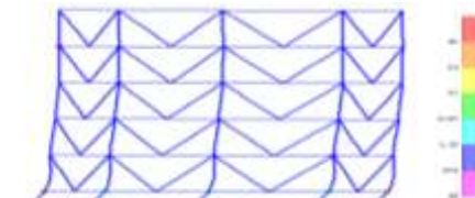
Fig. 12. Case (IV) V Braced Building
